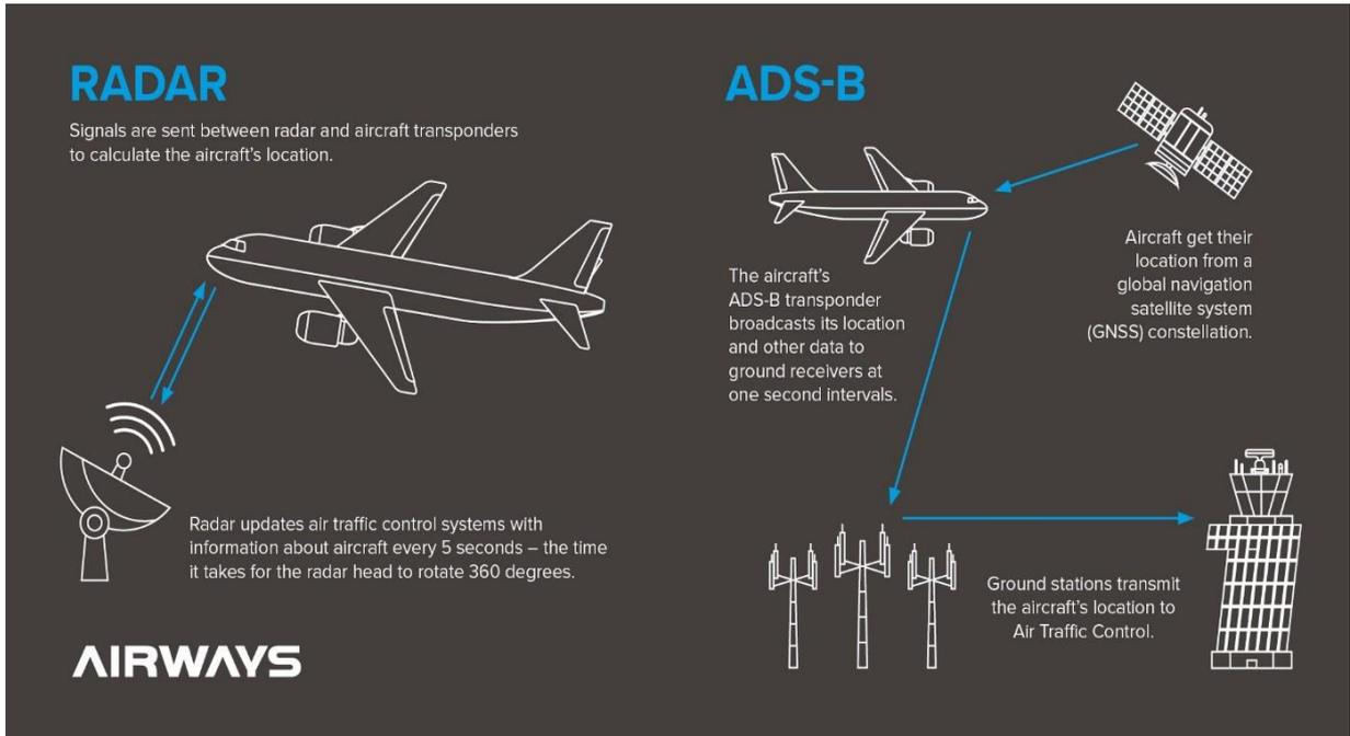
Figure 2 provides a functional overview of an aircraft ADS-B system
