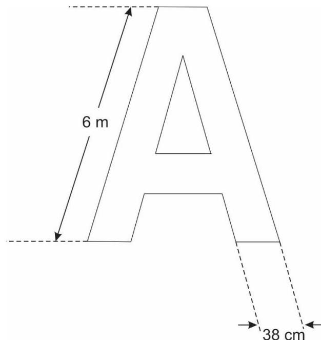
**Figure 1.** Agricultural operations aerodrome ground signal
